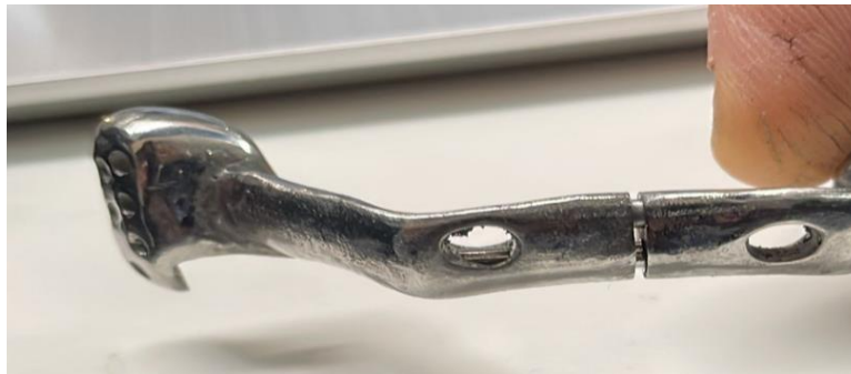
Figure: 4 Device manufactured with a sliding system to allow growth, and openings to allow tissue and muscle integration
