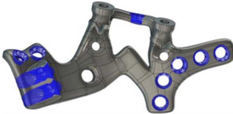
Figure 3: Constrictions for the Implantize Compact.
